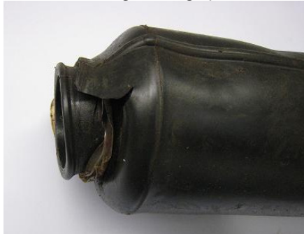
Figure 4 – RGD damaged pump system compensation bladder
