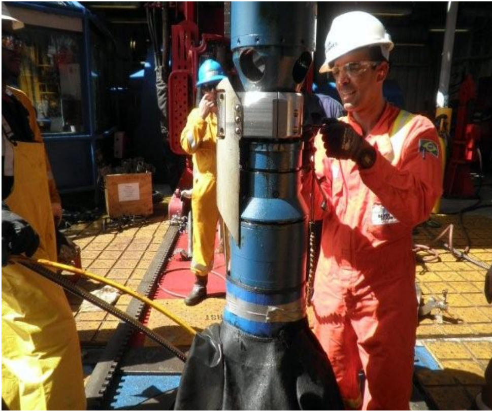
Installing the vibration clamp at the ESP pump intake.
